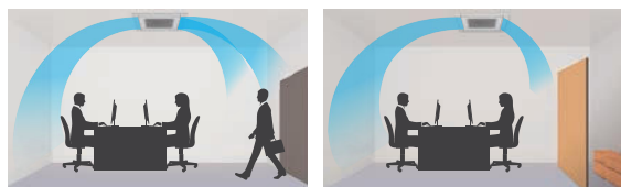
Comfortable air conditioning by preventing direct blowing of cold air and by providing swinging air flow simultaneously.
